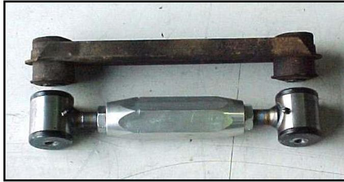
If the Hotchkis arm does not match the center-to-center length of the stock arm then you should adjust the length to match. Loosen the jam nuts at each end and turn the **center** section only! **Do not** turn the ends individually, as this will shorten the range of adjustment for the arm. Loosely tighten the jam nuts against the center section to hold it in place for the installation.
