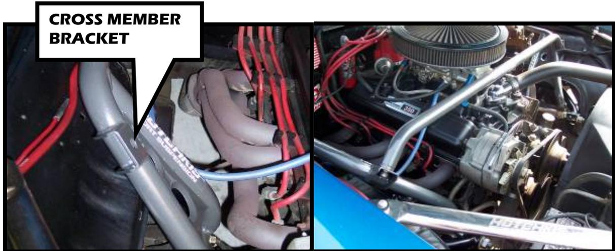
9. Now tighten the fender/firewall bracket end first and then tighten the A-arm bracket. Your Handle Bar Brace system is now ready to go.
