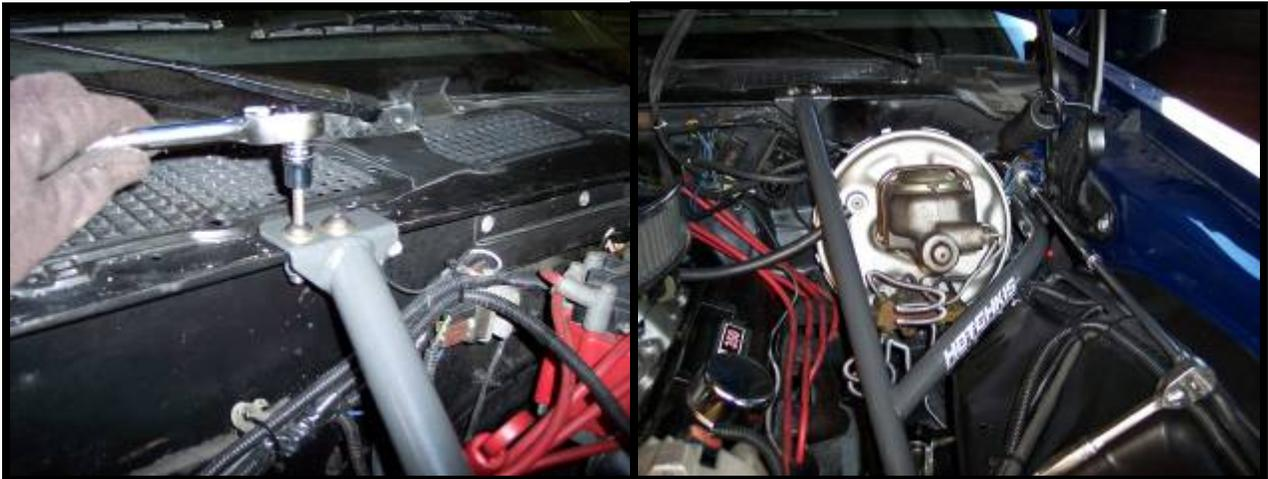
9. Finally, tighten the A-arm nuts. Perform these same steps on the other side and your Front Handle Bar Brace is ready to go.
