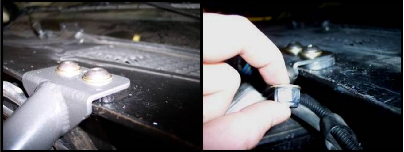
8. Tighten top firewall mount bolts and the fender bracket bolt.
