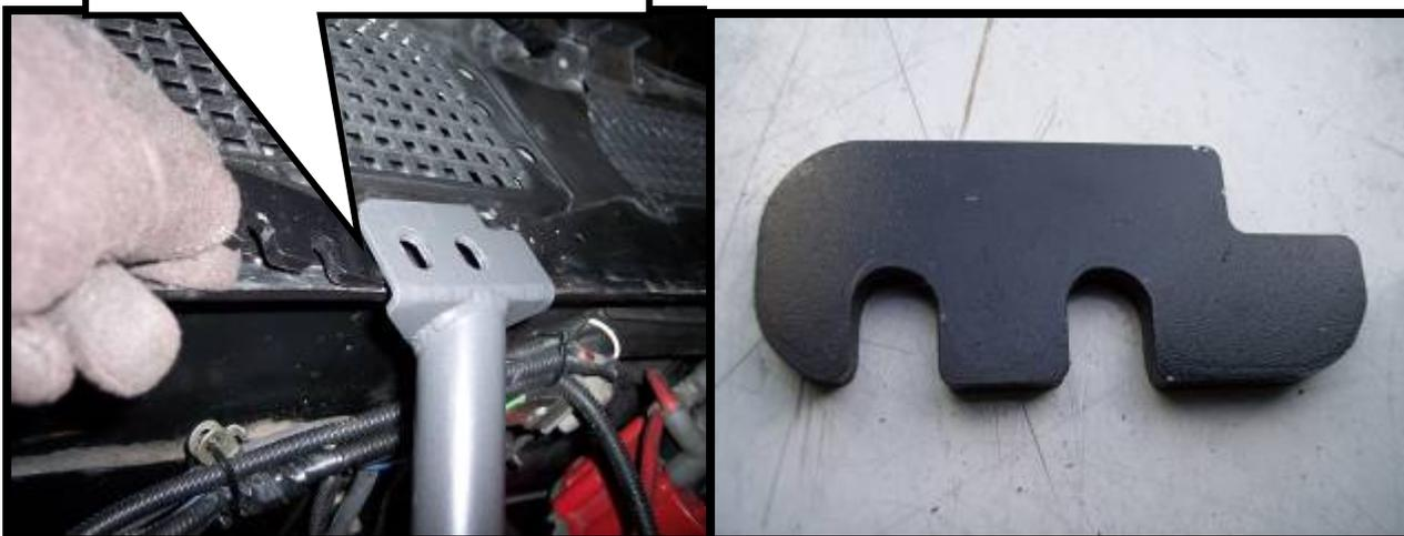
7. Using the provided hardware, place a 3/8" bolt with a washer into the top firewall mount. On the underside place a washer and a nylon lock nut on the bolt.
