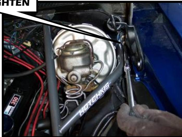
5. With the Handle Bar Brace now in place the holes for the top mount on the firewall can now be drilled. Once the first hole has been drilled place a bolt in that hole while drilling the second to ensure the Brace does not move.
