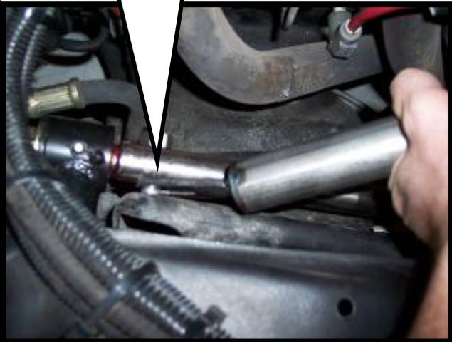
4. Put in the bolt that attaches the Handle Bar Brace to the fender bracket. Only tighten this bolt until it is snug, still allowing the Handle Bar Brace to move slightly.
