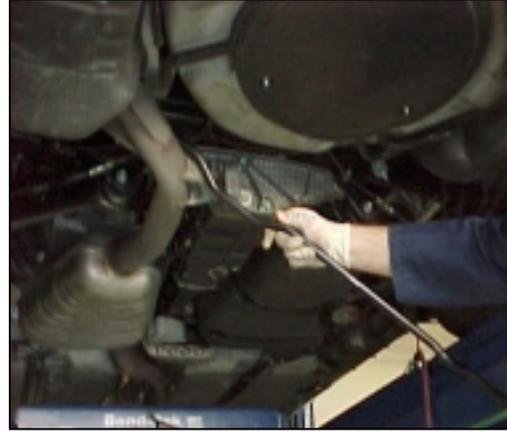
5/ Now install the reinforcement brackets. The **driver's side** frame has two holes above the rear portion of the lower a-arm. Use the flange-headed bolts and place the head on the inside of the frame facing out. Take the black bracket marked '**D**' and place it up against frame as shown. The '**D**' sticker will end up against the frame, with the gusset towards the ground. Use the lock washers and lock nuts provided. Assemble with 14mm wrenches **and leave loose, DO NOT TIGHTEN.**
