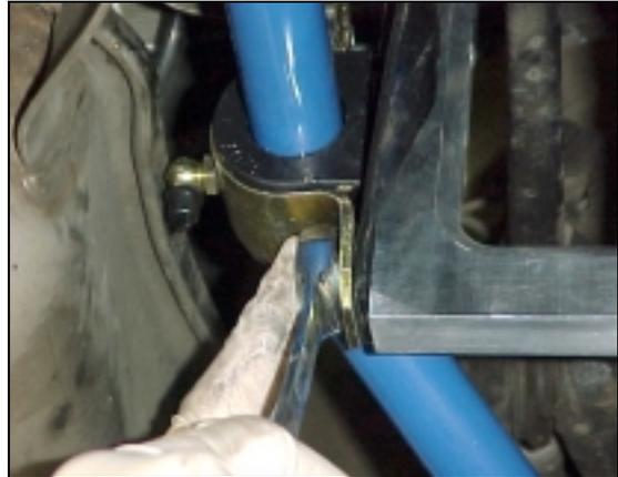
12/ Finally, choose the 'soft' or 'hard' setting for the end links and reinstall the nuts using the 16mm wrench and 5mm allen.
