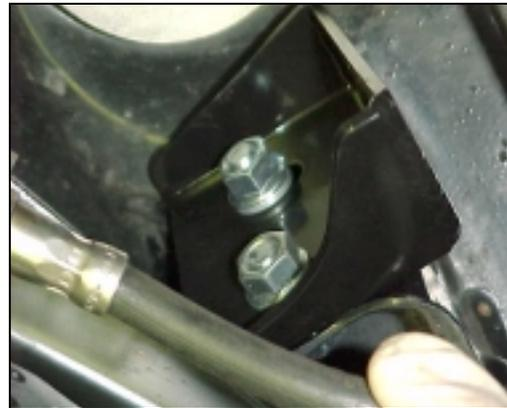
6/ Take one of the supplied billet pieces and remove one of the bolts. This allows you to open the piece and slide over the driver's side toe link. Reattach the bolt and washer (13mm wrench) **with the HSport sticker pointing towards the outside of the vehicle and tighten both bolts.** You may angle the brace up against the toe link itself to get enough leverage to tighten the bolts
