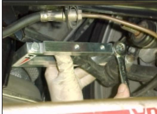
7/ Using the (2), 8mm x 20mm bolts and washers, attach the billet piece to the black bracket (13mm wrench) but DO NOT TIGHTEN. The black bracket is slotted, so use the slots to maneuver the pieces in order to thread the bolts.
