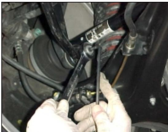
4/ Remove the four bracket bolts and nuts. Slowly remove the bar by rolling it over the exhaust. **WAIT TO INSTALL HSPORT BAR.**
