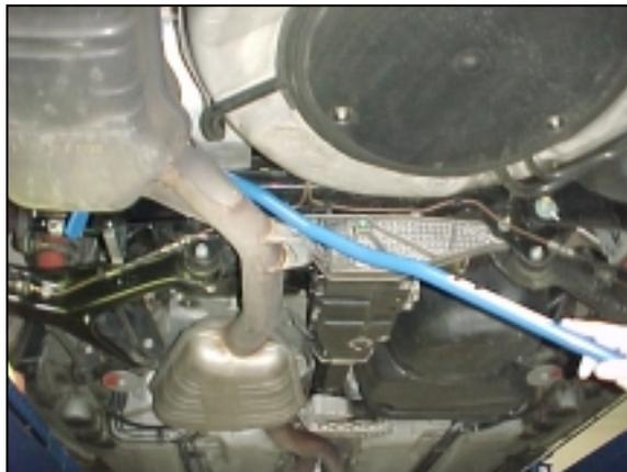
10/ Grease the inner portion of the smaller provided bushings using about one-quarter of the supplied grease pack. With the bar in, at the approx. stock location, install the smaller provided bushings in the approx. stock location. Then, install the bushing brackets with the grease fittings pointing down to the ground.
